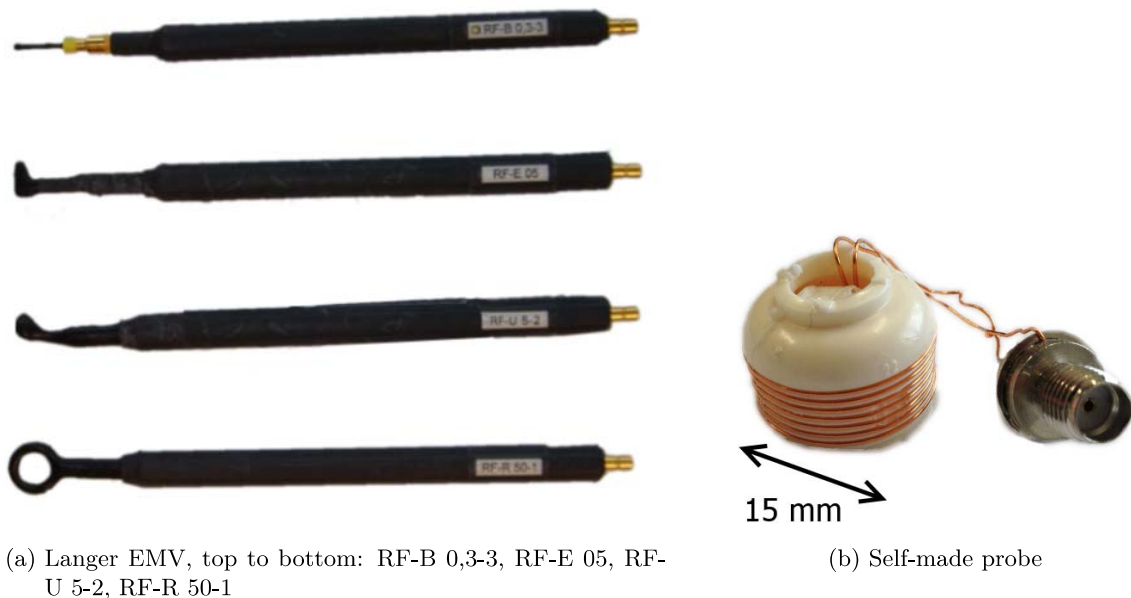
Figure 3.4: EM probes: Commercial set of probes by Langer EMV and custom probe made using copper wire
