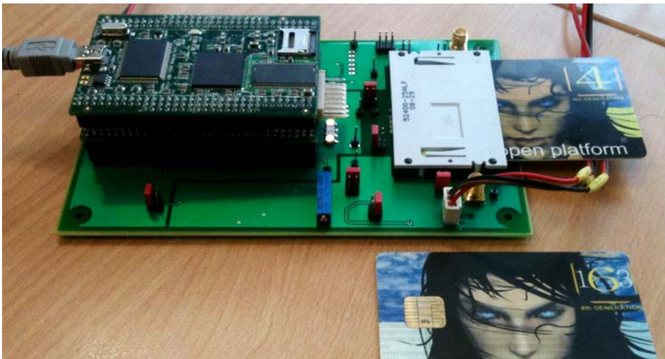
Figure 5.1: The GIANt with an ATmega-based smartcard
