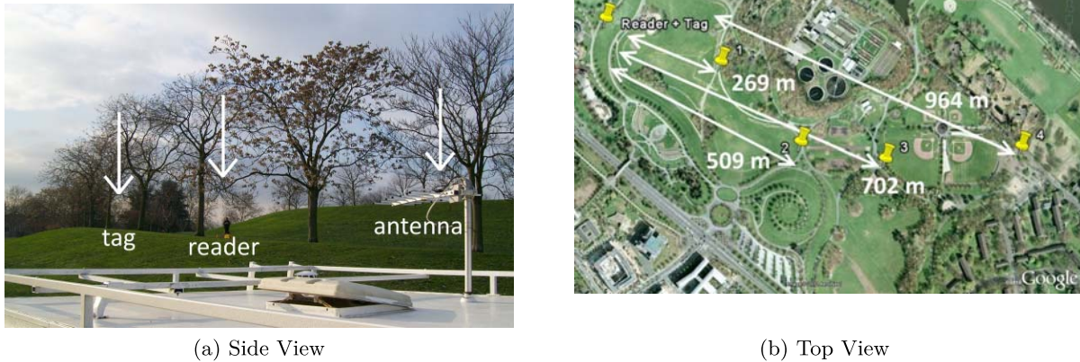
Figure 6.8: Setup and GPS coordinates for passive eavesdropping and detection
