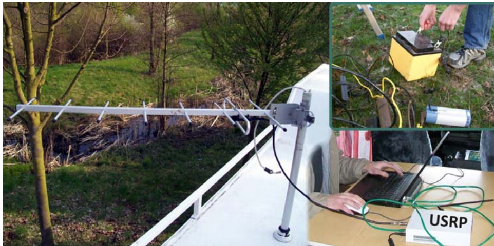
Figure 6.6: Mobile eavesdropping equipment. Left: Yagi-Uda antenna, connected to the data acquisition unit consisting of laptop and USRP2 in the measurement vehicle (right bottom); right top: voltage converter and car battery for the power supply in the wild
